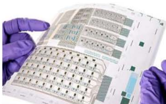
FIGURE 2.14 – Exemples de circuits flexibles.
