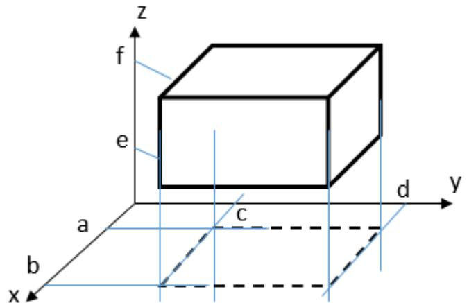
$$S = \iiint_{\Delta} 1 dx dy dz = \int_a^b \left[ \int_c^d \left[ \int_e^f 1 dz \right] dy \right] dx = (b - a)(d - c)(f - e)$$
