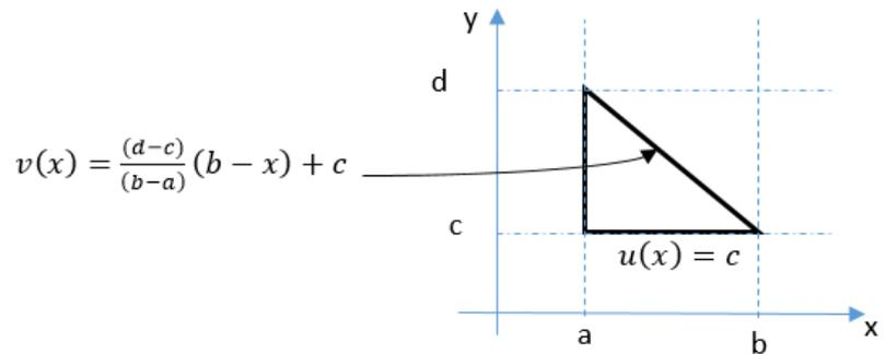
$$S_{tri} = \iint_D 1 \, dx \, dy = \int_a^b \left[ \int_{u(x)}^{v(x)} 1 \, dy \right] dx = \int_a^b \left[ \int_c^{\frac{(d-c)(b-x)+c}{(b-a)}} 1 \, dy \right] dx$$
