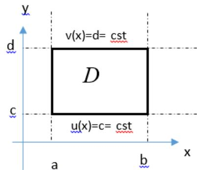
$$S_{rec} = \iint_D 1 dx dy = \int_a^b \left[ \int_{u(x)}^{v(x)} 1 dy \right] dx = \int_a^b \left[ \int_c^d 1 dy \right] dx = (b-a)(d-c)$$
