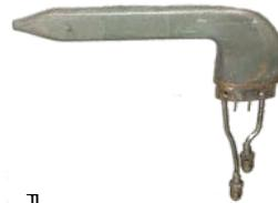
$$\left. \begin{aligned} p_3 &= p_2 + \frac{\rho v_1^2}{2} \\ p_2 &\approx p_1 \\ p_3 &= p_2 + \rho_{man} gh \end{aligned} \right\} \Rightarrow v = \sqrt{\frac{2\rho_{man} gh}{\rho}}$$
