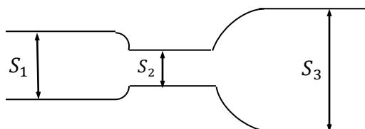
$$Q_V = S_1 v_1 = S_2 v_2 = S_3 v_3$$
