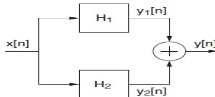
$$y(n) = y_1(n) + y_2(n) = H_1[x(n)] + H_2[x(n)] = [H_1 + H_2]x(n) = H_P[x(n)]$$
