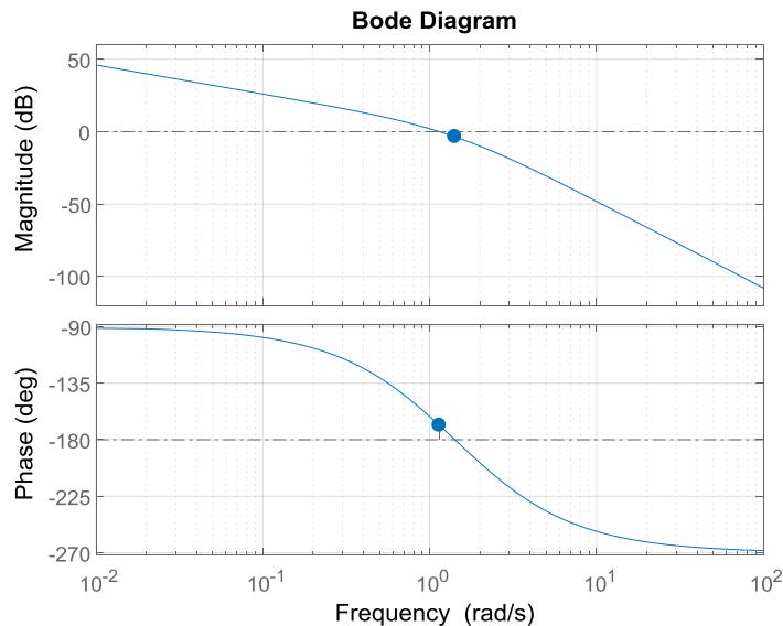
$$\begin{aligned} \omega_{c0} &= 1.14 \text{ rad/s} & M\varphi_1 &= 11.4^\circ \\ \omega_{-\pi} &= 1.41 \text{ rad/s} & MG_1 &= 3.52 \text{ dB} \end{aligned} \rightarrow \text{système stable}$$
