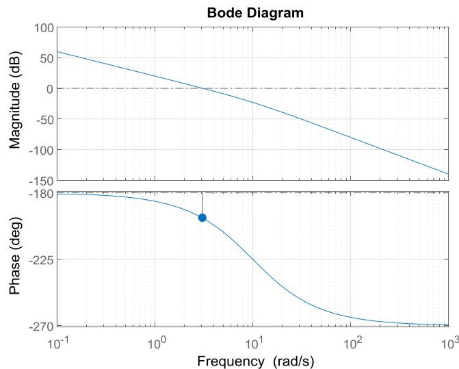
$$\begin{aligned} \omega_{c0} &= 3.09 \text{ rad/s} & M\varphi_1 &= -17.2^\circ \\ \omega_{-\pi} &= 0 \text{ rad/s} & MG_1 &= 0 \end{aligned} \rightarrow \text{système instable}$$
