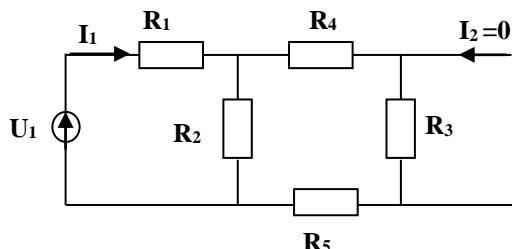
$$R_{eq} = R_1 + \frac{R_2 (R_3 + R_4 + R_5)}{R_2 + R_3 + R_4 + R_5} = Z_{11}$$
