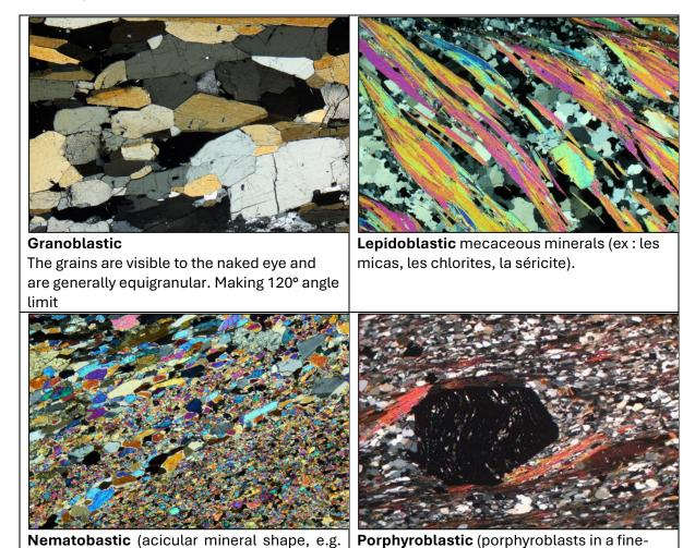
Porphyroblastic (porphyroblasts in a fine-
