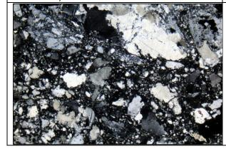
**Mylonitic or cataclasic** (Minerals are ground and crushed)
