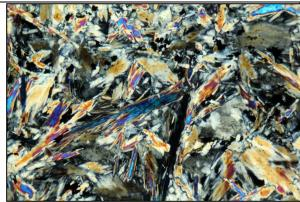
**Decussate or diablastic** (interlocking but not overlapping minerals. The grains are medium to coarse (crystals > 0.5 mm),
