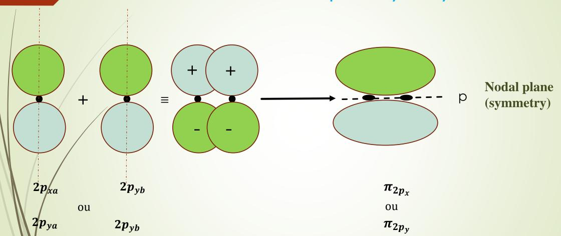
$\pi$ -orbital: molecular orbital (MO) resulting from the lateral overlap of two p orbitals with a nodal plane passing through the bond axis.
