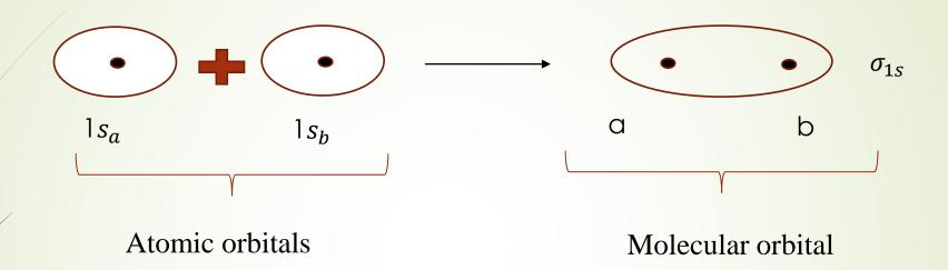
$\sigma_{1s}$  Cylindrically symmetric about the bond axis.
