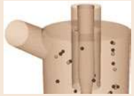
V3.4 Hydrocyclone separator
