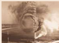
V3.5 Aircraft wing tip vortex
