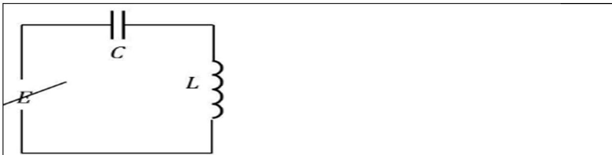
$$E_c = E_{mag} = V_L dq = \int L \frac{di}{dt} dq = \int L i di = \frac{1}{2} L i^2 = \frac{1}{2} L \dot{q}^2$$
