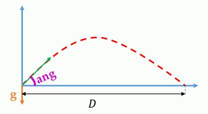
$D = (speed^2 \times \sin(2 \times angle))/gravity$
