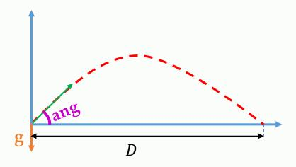
$D = (speed^2 \times \sin(2 \times angle))/gravity$
