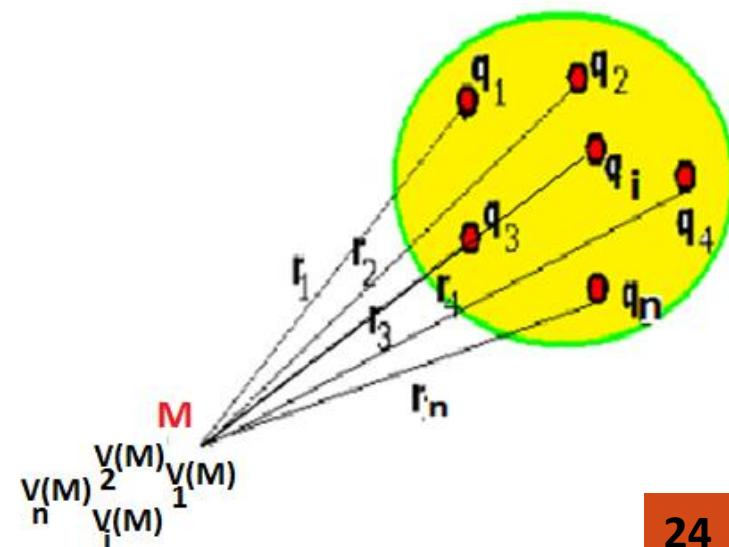
$$\begin{aligned} V(M) &= \sum_{i=1}^n V_i(M) = \sum_{i=1}^n K \cdot \frac{q_i}{r_i} = K \cdot \sum_{i=1}^n \frac{q_i}{r_i} \\ &= V_1(M) + V_2(M) + \cdots + V_i(M) + \cdots + V_n(M) \end{aligned}$$
