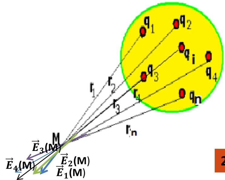
$$\begin{aligned}\vec{E}(M) &= \sum_{i=1}^n \vec{E}_i(M) = \sum_{i=1}^n K \cdot \frac{q_i}{r_i^3} \vec{r}_i = K \cdot \sum_{i=1}^n \frac{q_i}{r_i^3} \vec{r}_i \\ &= \vec{E}_1(M) + \vec{E}_2(M) + \dots + \vec{E}_i(M) + \dots + \vec{E}_n(M)\end{aligned}$$
