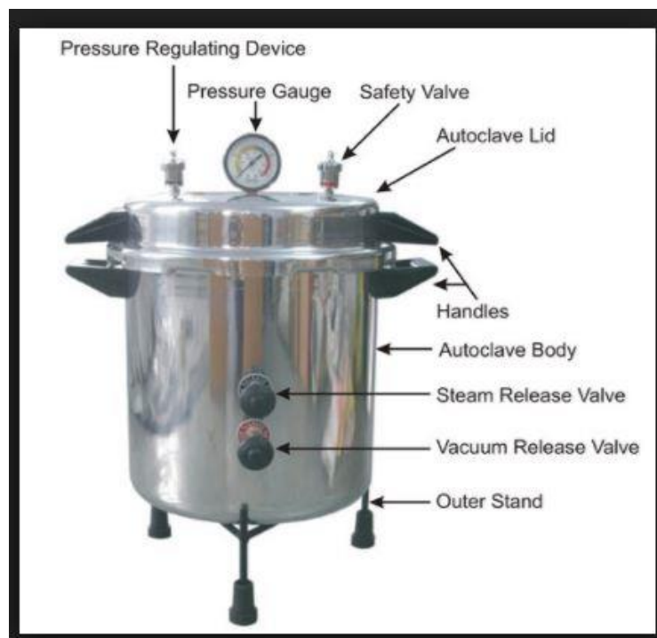
Figure 5. Example of a standard benchtop autoclave (Fund, 2018).
