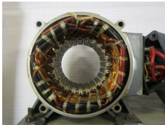
Figure IV.9: Winding location in a stator core
