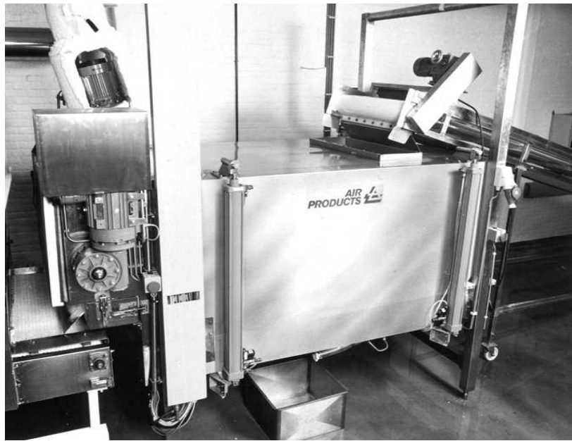
Figure 13. Immersion freezers use a bath of liquid nitrogen (Butcher and Copy, 2000).
