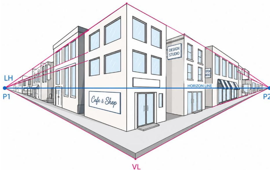
Figure I. 14: Conical oblique perspective
