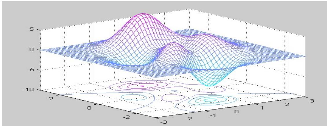
The command *meshz* generates the curtain plot for the peaks function:
