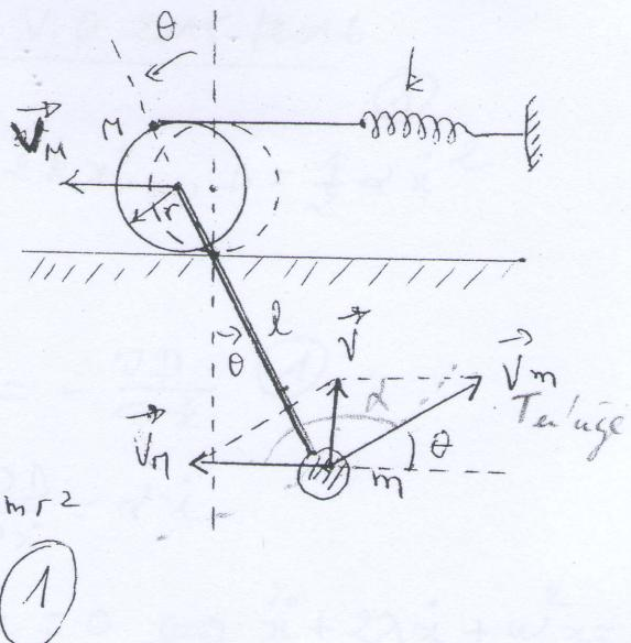
~~$$1) \quad E_C = \frac{1}{2} m \dot{x}^2, \quad E_P = \frac{1}{2} k (x+x_0)^2 - \frac{1}{2} k x^2, \quad D = \frac{1}{2} \alpha \dot{x}^2$$~~
