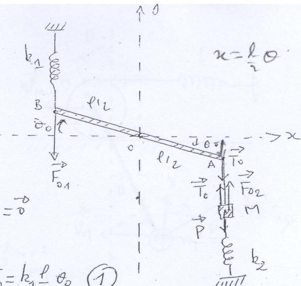
$$\text{base: } \sum \vec{F}_{\text{ext}} = \vec{0} \Rightarrow \vec{F}_{02} + \vec{P} + \vec{T}_0 = \vec{0} \Rightarrow T_0 = Mg - k_2 \frac{l}{2} \theta_0 \quad (1)$$
