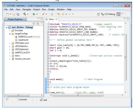
Right click on Project name in the Project Explorer > Show Build Settings > Build > C6000 Compiler > Processor Options > Target processor version and set its value to "6713" (no quotes)
