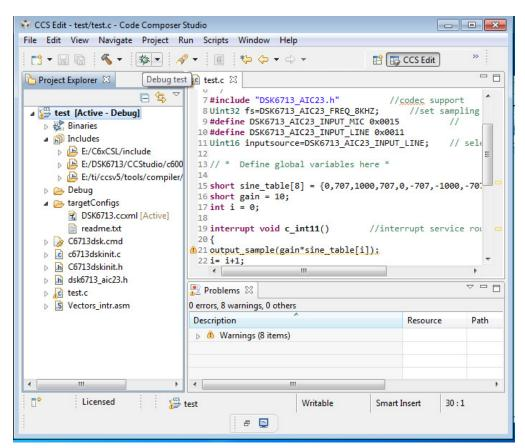
This will load the .out file (ie executable code) to be loaded into the DSK.
